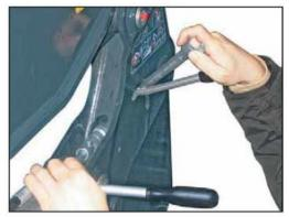
To set the lock, you will need an open-ended spanner (WAF 24), a ½" ratchet with the corresponding extension, joint and 24 mm socket spanner.
